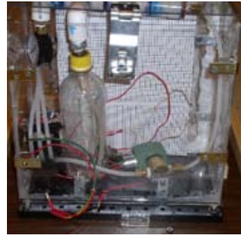
Complex plumbing in a DIME 2003 experiment for water streams in microgravity
