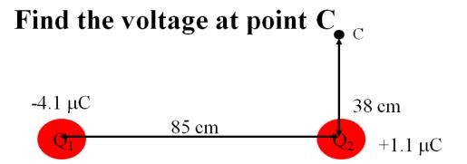
The work done to move a point charge is  $W = q\Delta Ve$ , where  $\Delta Ve = Vf - Vi$
