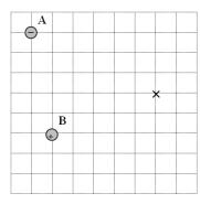
Charge A is -1.20  $\mu$ C, charge B is +3.40  $\mu$ C Find the Potential at the x (Each square is a meter)
