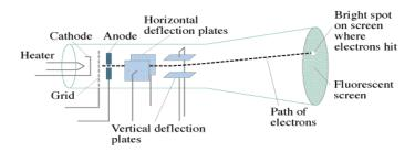
Part 1 - Acceleration toward the anode:  $Ve = {}^{1}/_{2}mv^{2}$ Example - A CRT uses an accelerating potential of 5200. V. What velocity do the electrons have when they pass through the anode?
