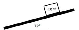
A 5.0 kg object is on an inclined plane that makes an angle of  $26^{\circ}$  with the horizontal. Make up the plane positive. The coefficient of kinetic friction is 0.35, and static is 0.52 A) What are the components of gravity parallel and perpendicular to the plane? What is the force of
