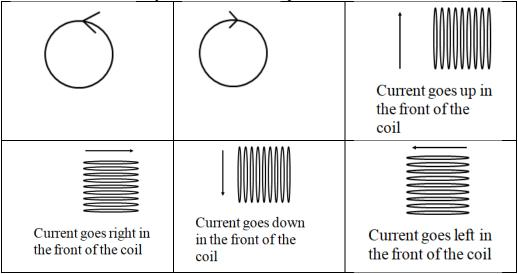
2. The direction the current flows in the loop or solenoid due to a change in flux: (three steps) Find the direction of the change of flux. Are you gaining or losing flux, and which way is it?
