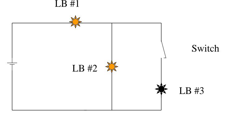
When the switch is open (no current flows through it) light bulbs 1 and 2 burn with equal brightness.
