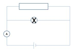
**3.** Consider the circuit below. Three equivalent light bulbs with a resistance of 7.20 ohms are connected as shown. The cell has a potential of 16.0 V and negligible internal resistance.
