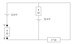
a. Calculate the current through the 6, 8, and 17  $\Omega$  resistors (0.259 A down, 1.06 A up, 0.797 A left) b. What is the potential difference between X and Y? (1.55 V)
