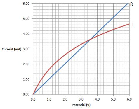
a. Explain whether the light bulb or the resistor can be said to be Ohmic.
