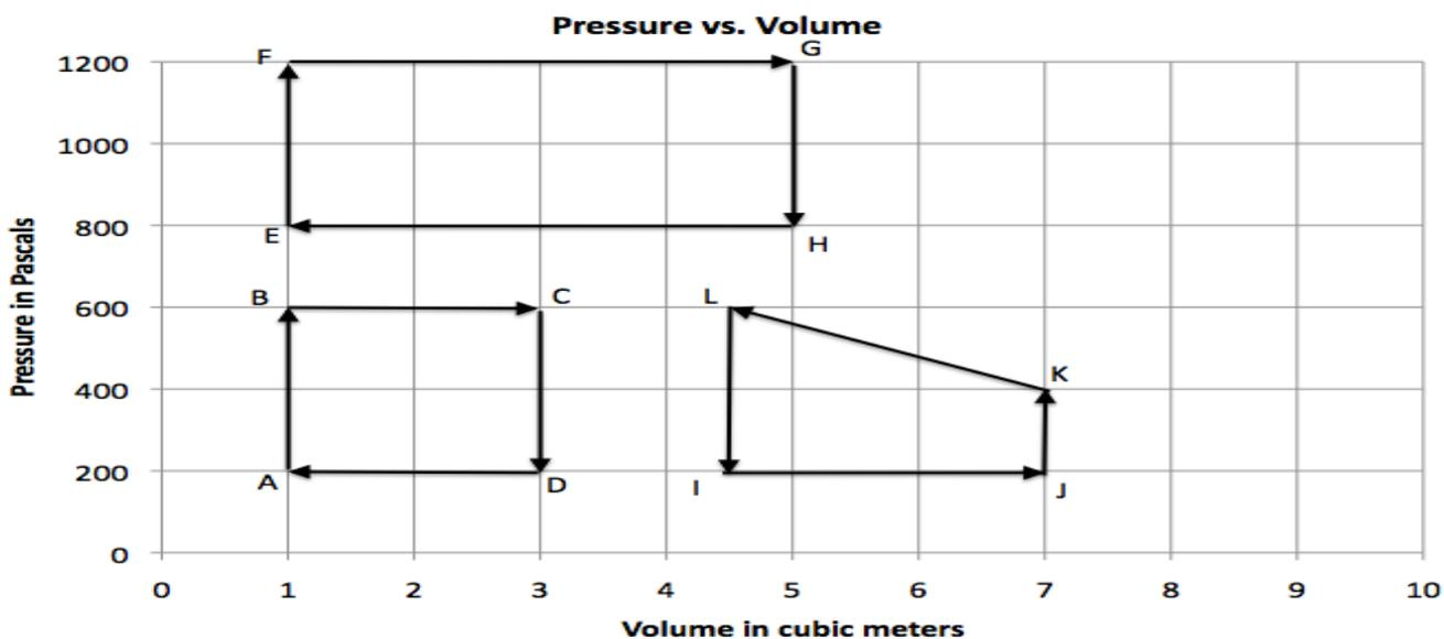
26. What is the net work done for cycle ABCD? If point A is at 60.0 K, how many mols of gas do you have, and what are the temperatures of the other vertices BCD, (+800 J, 0.401 mols, 180 K, 540 K, 180 K)
