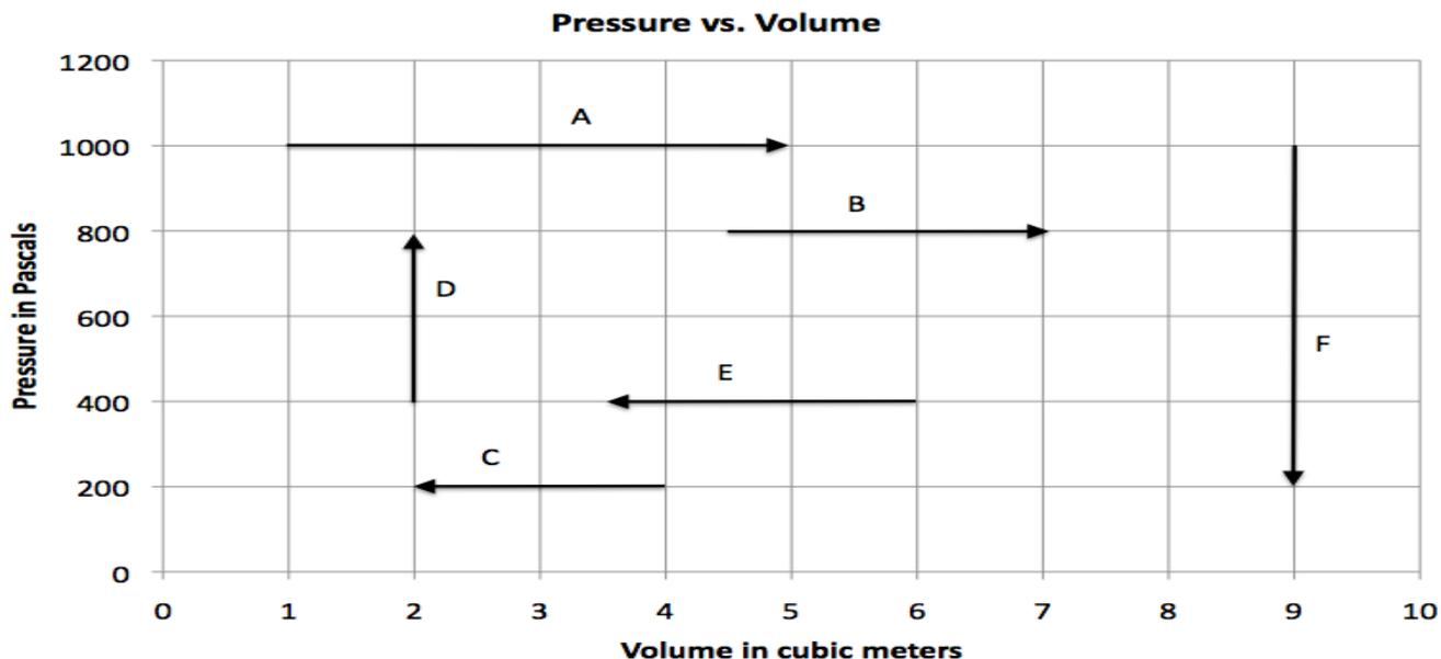
For each process, calculate the work done, and say what happens to the pressure, volume and temperature.
