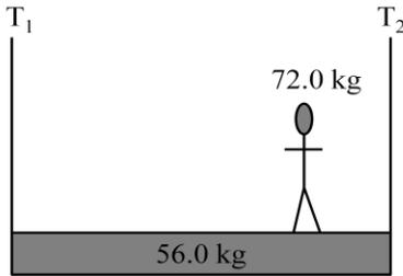
2. The beam is 11.0 m long, and the person is standing 4.00 m from the left side. Find the forces exerted by the supports.
