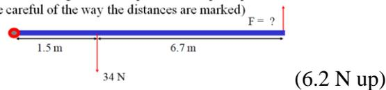
Find the missing Force. Torque about the pivot point.
