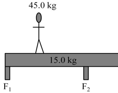
5. The beam is 12.0 m long, the second cable is attached 7.00 m from the left side, and the person is standing 4.00 m from the right side. Find the tensions in the cables.
