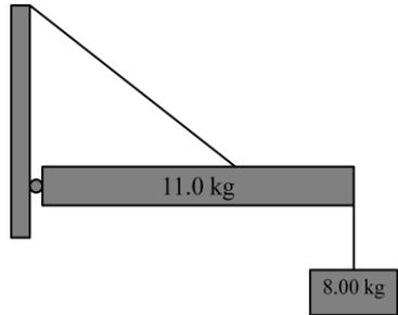
8. The cable makes an angle of  $25.0^\circ$  with the 16.0 m long beam. The sign hangs 5.20 m from the left side of the beam. Find the tension in the cable, and the horizontal and vertical components of the force exerted by the wall. Be sure to give the direction of the components.
