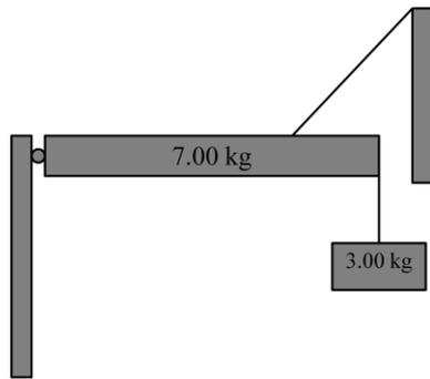
12. The rod is connected 3.20 m from the left side of, and makes an angle of  $38.0^\circ$  with the 4.00 m long beam. The box is centered 1.20 m from the left side. Find the force along the rod, and the horizontal and vertical components of the force exerted by the wall. Be sure to give the direction of the components.
