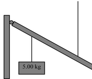
11. The cable is connected 1.50 m from the left side, and makes an angle of  $48.0^\circ$  with the 2.00 m long beam. Find the tension in the cable, and the horizontal and vertical components of the force exerted by the wall. Be sure to give the direction of the components.
