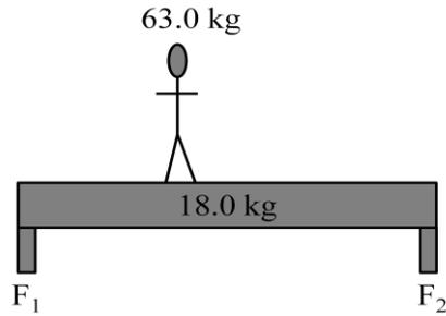
3. The beam is 8.20 m long, and  $F_2$  is 3.00 m from the left side, and the person is 0.500 m from the right side. Find the forces exerted by the supports.
