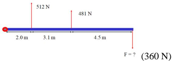
Find the missing force. Torque about the pivot point.
