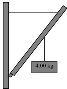
10. The cable is connected 10.0 m from the hinge, and makes an angle of  $60.0^\circ$  with the 12.0 m long, 8.00 kg beam. The sign hangs 3.10 m from the hinge. Find the tension in the vertical cable, and the horizontal and vertical components of the force exerted by the wall. Be sure to give the direction of the components.
