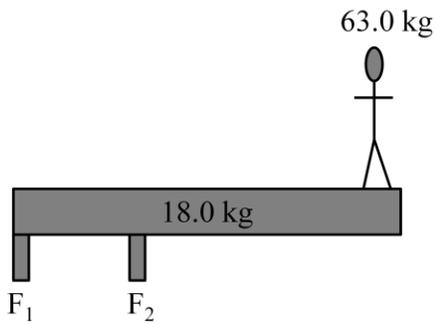
4. The beam is 9.00 m long, and  $F_2$  is 3.00 m from the right side, and the person is 3.00 m from the left side. Find the forces exerted by the supports.
